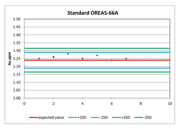
Figure 11.8 Analyses of Standard OREAS-66A
